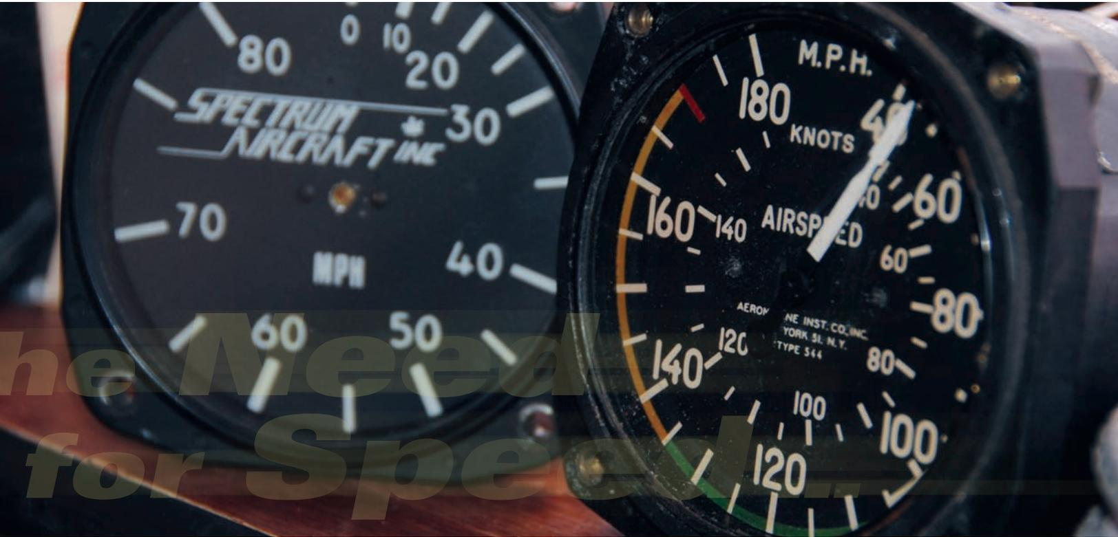
source. The airspeed indicator then displays this pressure difference to the pilot as IAS.
