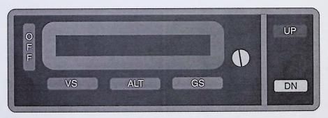
Fig. 2-2. AP Display, All Annunciations Extinguished
